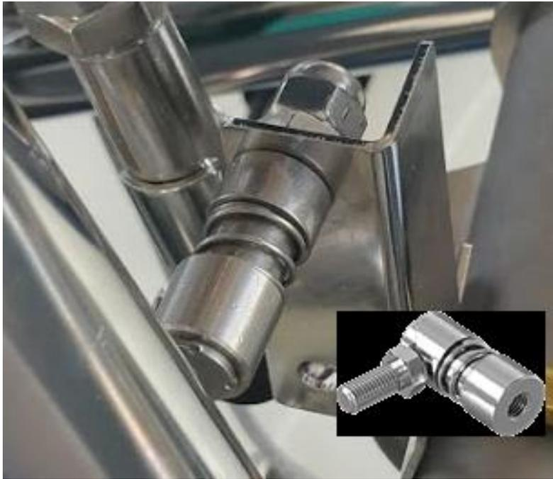
The ball joints are  $\frac{1}{4}$ "-28 threaded on both ends. When securing them it is highly recommended that Loctite thread locker be used. An alternative would be 3M 5200.
