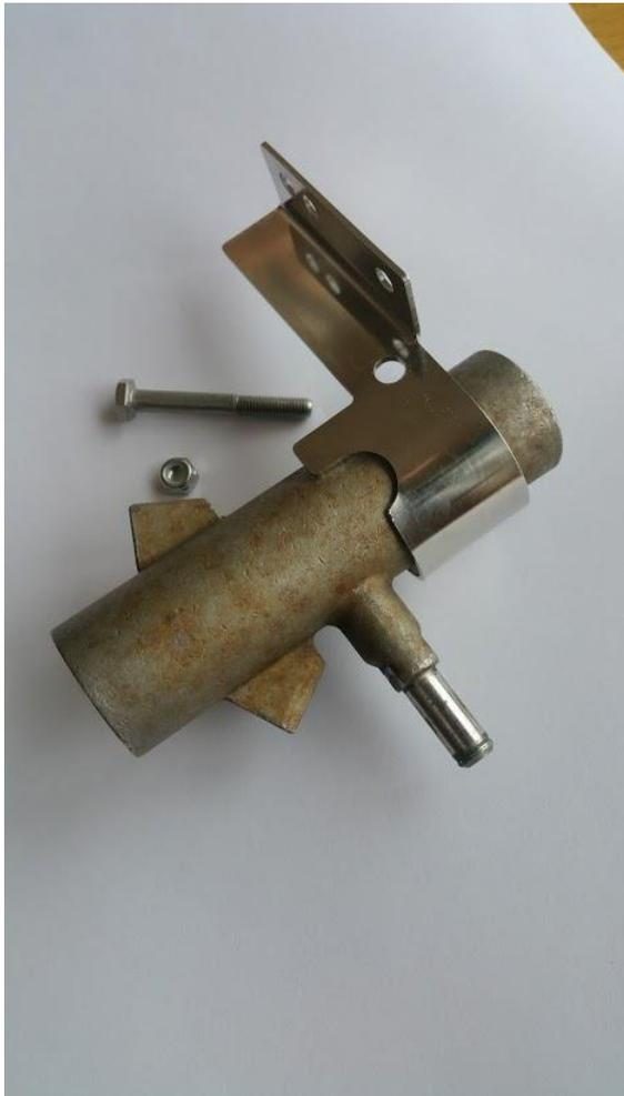
Attaching the WV pinion bracket. Slide it onto the pinion gear then tighten the bolt and nut combination. The bracket locks onto the pinion gear and the wind link arm.
