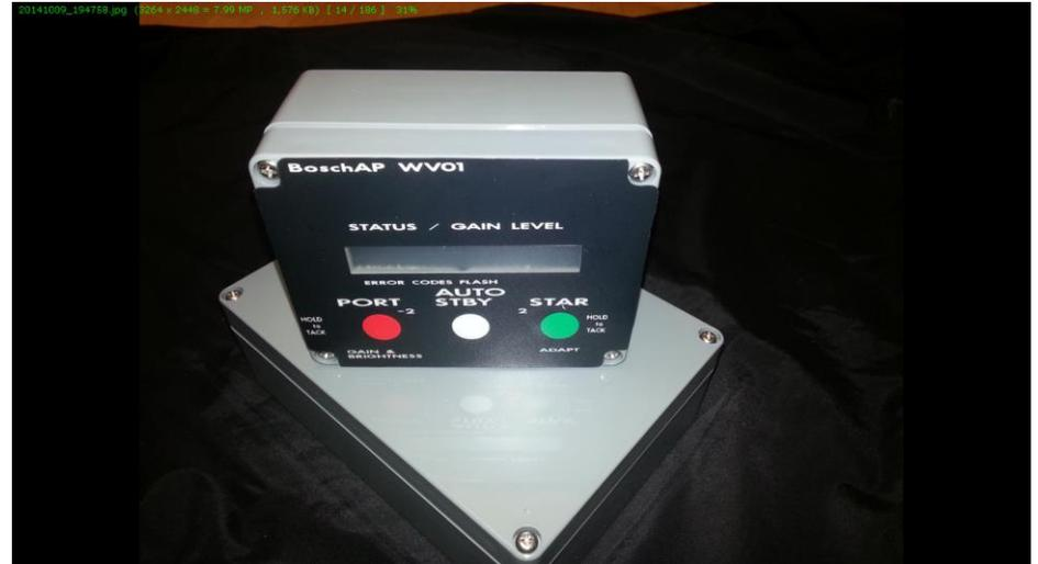
Original model: The USB connector is Exposed by removing the 4 screws On the front panel and then removing the circuit board with the 3 screws holding it in place.
