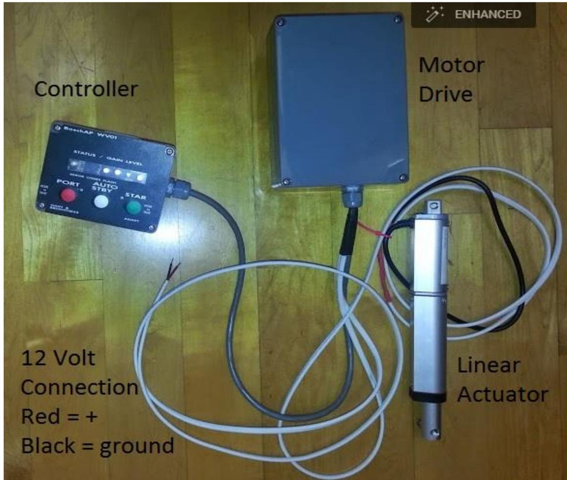
Actuator shown is for windvane control.
