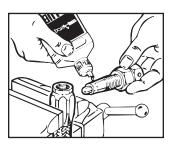
**Step 3**. *Male Ends:* Push assembly tool into nipple.
