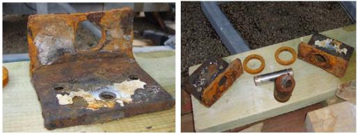
The nylon parts and the original stainless steel pivot pin were all in perfect condition which makes me think that all the pivoting has been between the stainless steel pin and the mild steel brackets. I had to cut the nylon bearing through the keel as it wouldn't budge. The pivot hole through the keel was sound with no rust. I also decided to fit a zinc anode to help protect against future rust.
