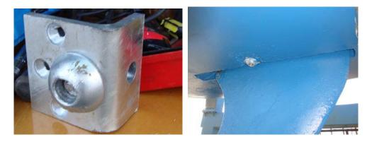
I painted the pivot holes on the angle brackets before inserting the new pin and greased the main nylon bearing to ensure that the pivoting would be in the correct place in future. I used plenty `Sikaflex marine sealant 291' to ensure a good seal around the bolts.
