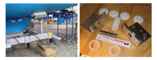
The job was reasonably straight forward but the new bracket holes didn't align correctly which was a bit of a pest to say the least! CHECK THE HOLE ALIGNMENT BEFORE APPLYING ANY MASTIC! The brackets were ordered from Beneteau and £50 a piece. They are 10mm galvanised mild steel (not Stainless). If I did this again I'd have the new brackets fabricated in stainless.
