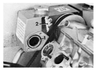
8. Pull the heat exchanger's fresh water section to one side. The fresh water section is mounted on a rubber bushing (1) and the water pipe (2), which seals against an O-ring.
