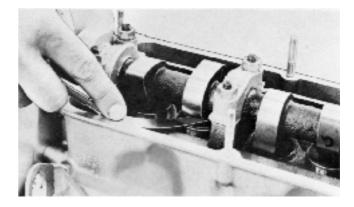
**136.** Fit the cover (with the firing position marking).
