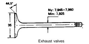
IMPORTANT! The valves have a stellite coating. Therefore, they are not to be cut or ground but only lapped into the seat.
