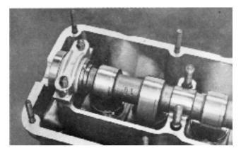
111. Fit tool 999 5021 and depress the camshaft.
