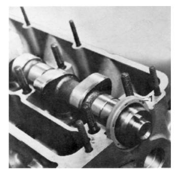
**34.** Fit tool 999 5021 on the camshaft. Use the bearing cap's nuts. The camshaft is held in position with the tool. Undo the other four camshaft bearing caps.
