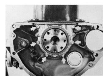
**53.** Remove the locking ring for the bearing on the input shaft.
