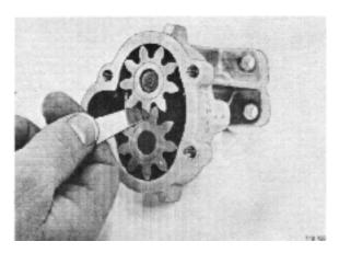
**84.** Check the axial clearance. The axial clearance is 0.02–0.12 mm (0.008–0.0047").
