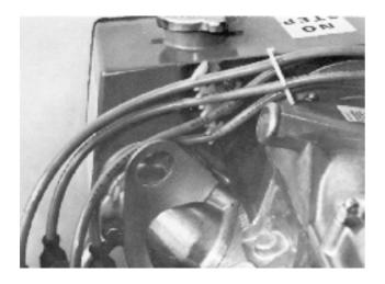
**165.** Fit the fuel pump. Use new gaskets. Fit the tensioning bar and the engine mounting with the bracket for the alternator. Then tighten the alternator in position and fit and tension the belt so that it can be depressed approximately 5 mm (0.2 in) with normal thumb pressure.
