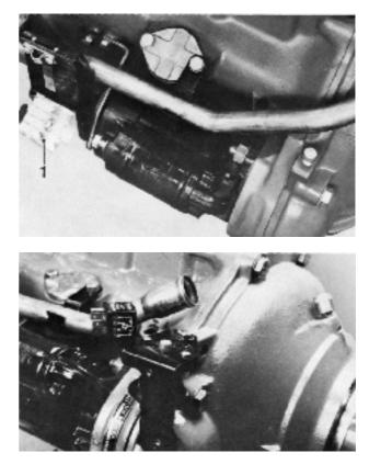
**167.** Fit the oil dipstick sleeve in the crankcase. NOTE! The bracket for the ignition coil is to be fitted on the flywheel cover's upper side in the existing screw holes. (Screw diameter 5/16 UNC length 19 mm) (3/4"). Then fit the ignition coil and the cable loom. Connect all the cables and clamp the cable loom in position.
