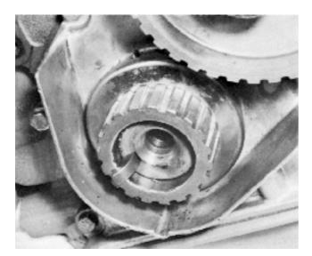
**28.** Unscrew the flywheel cover's four screws and the three screws which hold the protective plate on the underside between the cover and the cylinder block.
