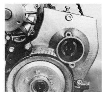
**139.** If the clearance is incorrect the adjustment shims are to be changed as follows: Turn the valve pusher so that the groove is at right angles to the camshaft's length.
