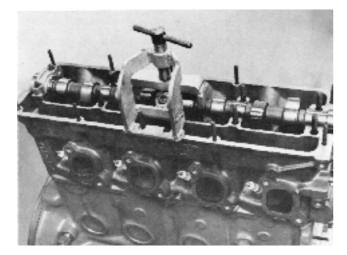
**113.** Oil and lay the other three bearing caps in position and fit the nuts for the four bearing caps. Tighten them somewhat NOTE! The forward bearing cap's surface against the cylinder head **is to be painted with sealing fluid** before it is fitted. Make sure that the seals fit correctly before the front bearing cap is tightened. Then remove the tool.
