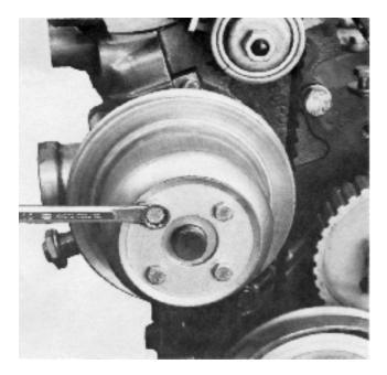
**19.** Remove the crankshaft pulley. Six screws. The spanner width is 10 mm.
