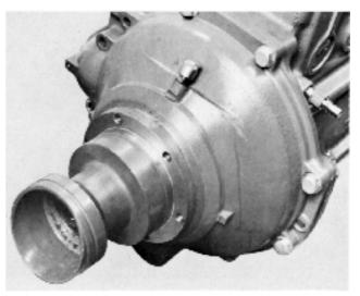
**29.** Remove the vibration damper's six screws. Spanner width 13 mm. Carefully remove the vibration damper from the three guide pins.
