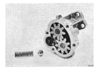
**83.** Refit the gear wheels and check the gear flank clearance which is 0.15–0.35 mm (0.0060–0.014").
