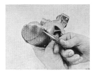
**85.** Lay the ball and the spring in position and refit the cover.
