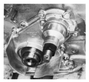
**120.** Paint mineral grease or similar grease in the flywheel's hub and replace the flywheel and the guide plate on the camshaft. The flywheel's groove is to be fixed on the guide pin on the camshaft. NOTE! The guide plate's bend is to point backwards (against the seal).
