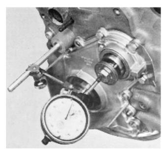
**116.** Push the intermediate shaft in carefully in the crankcase so that the intermediate shaft's gear wheel does not damage the bushings in the block. Use tool 999 4030.
