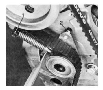
**129.** Turn the crankshaft clockwise a few degrees. This is to take up the backlash between the pulleys. NOTE! Do not turn the crankshaft anti-clockwise otherwise the belt can hop over teeth and alter the adjustment.
