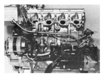
**168.** Lay the gaskets for the induction pipe in position. Fit the induction pipe with the lifting eye on the rear studs. Tighten the nuts with a torque of 20 Nm (2 kpm) (14.8 lbf. ft.). Fit the oil dipstick sleeve in the induction pipe.
