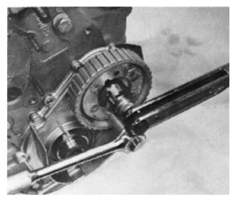
**123.** Paint mineral grease or similar lubricant in the hub on the crankshaft's pulley. Position the guide plate (turn the bend towards the seal) and fit the pulley on the crankshaft. Then refit the outer plate and the carrier and fit the screws. The tightening torque is 165 Nm (16.5 kpm) (122 lbf. ft.). Use a suitable counterforce.
