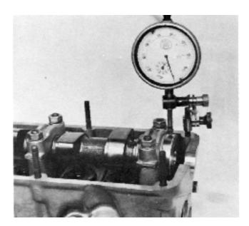
**48.** Replace the valve pressers in the cylinder head and check that the play is not too much or that they do not stick. The play between the valve pressers and the cylinder head is 0.030–0.075 mm (0.0012–0.0030").
