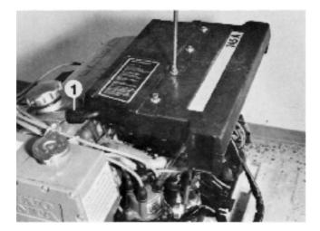
**3.** Remove the alternator, drive belt, cable harness, ignition coil, main fuse, starter motor, ignition cables and distributor. NOTE! Mark the cables before they are removed.
