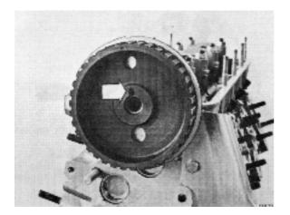
**122.** Paint mineral grease or similar lubricant in the pulley's hub and fit it in position on the intermediate shaft. Fit the screw and tighten it with a torque wrench.
