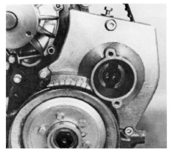
**17.** Remove the circulation pump's pulley. The spanner width is 10 mm.
