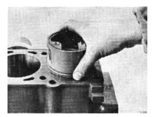
Measure the piston ring gap by rolling the piston rings in the groove. Check the play at several points with a feeler gauge. The play is: Compression rings: 0.040-0.072 mm (0.0016-0.0028") 0.030-0.062 mm (0.0012-0.0024") Oil scraper ring:
