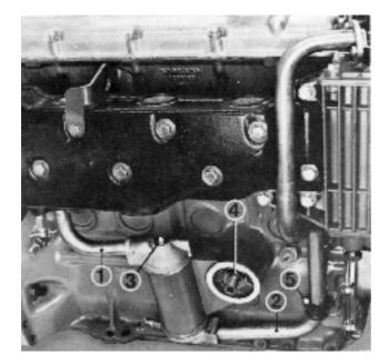
**15.** Remove the saltwater pump and the generator's tensioning bracket. The spanner width for the saltwater pump is 10 mm. The other screws which hold the cover have a spanner width of 8 mm. Check the impeller, the key and the packing on the pump's front side plus the sealing ring on the pump's rear side. Clean the pump and replace damaged parts.
