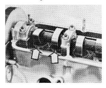
141. Remove the shim with pliers 999 5026.
