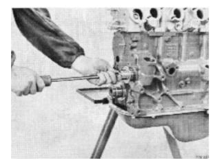
**118.** Fit the crankshaft seal with tool 999 5024. Lubricate the seal's rubber lip before fitting. If the spacer tube on the crankshaft has not been removed the position for the sealing ring is to be changed so that a new contact surface against the tube is obtained. Be careful when fitting the seal so that the rubber lip is not damaged and that the spring does not jump out of position.
