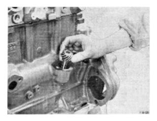
**134.** Fit the cover and the brackets for the cooling water pipe. NOTE! Check first that the cover's pressure surface (which presses against the oil pump drive) is not worn.
