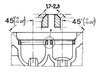
**43.** Check that all the valves and the valve seats are perfectly ground by marking the valve seat face and turning it against the valve seat with light pressure. If the marking is not evenly distributed on the whole of the seat (leaking valve) the valve is ground further and a new check is carried out until the result is satisfactory.
