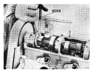
**140.** Fit tool 999 5022 and depress the valve pressers. Screw the tool spindle down and adjust its length so that the presser's groove lies over the edge and is accessible with the pliers.
