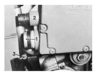
**160.** Fit the ingoing and outgoing cooling water pipes to the salt water pump and press the ingoing pipe into the bracket (1).
