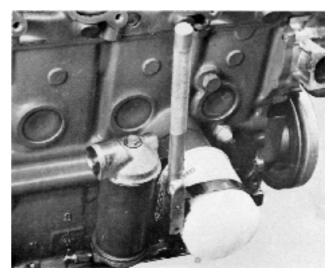
**13.** Remove the nut (1) and remove the oil cooler. Only AQ145. Spanner width = 28 mm. Remove the oil pressure
