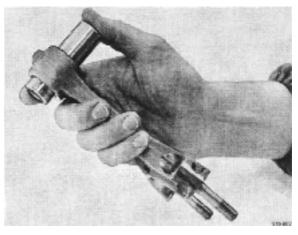
**76.** Check the connecting rods for straightness, torsion and possible s-bends. Use a connecting rod straightener. Nuts and screws are to be replaced when overhauling.
