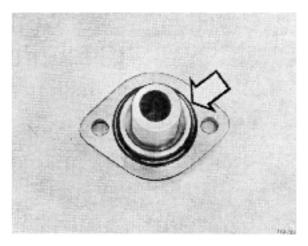
**132.** Fit the oil pump drive. It is possible that the crankshaft (intermediate shaft) may need to be turned somewhat so that the oil pump drive engages.
