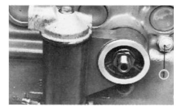
**155.** Place the screws in the exhaust pipe and hang the gasket in position. NOTE! The marking "UT" is turned outwards. Then fit the pipe to the engine. A lifting eye is fixed with one of the screws.
