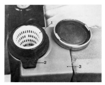
6. Remove and discard the O-ring (1) in the heat exchanger and if necessary, unscrew the holder (2) for the ignition cables. The holder is fixed with two guide pins.
