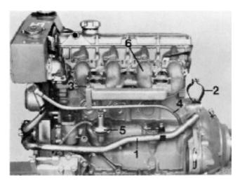
Remove the thermostat housing and lift out the thermostat.
