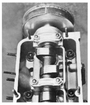
**138.** Measure the valve clearance with a feeler gauge for No. 1 cylinder.
