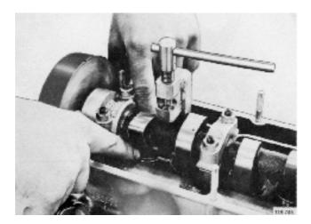
**146.** Check the clearance for all the valves. NOTE! Turn the camshaft a few times before checking.
