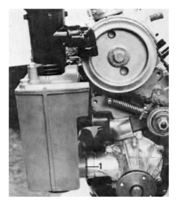
**158.** Oil the lubricating oil filter's rubber packing and screw the filter in sufficiently so that the rubber packing just comes into contact with the engine body. Then screw it another half turn by hand. Check the oil pressure and for leakage around the oil filter during the first test run.
