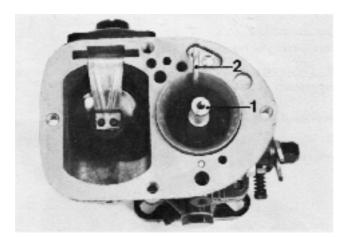
**93.** Rotate the throttle shaft (1) and press out the push rod (2) from the lever (3). Then rotate the push rod downwards and disassemble the check valve (4). Blow the check valve clean and the strainer. Clean and blow the carburetor and its ducts. Then re-fit the check valve and strainer. NOTE! Do not forget the copper washer. Rotate the throttle shaft somewhat and press the push rod into the lever.
