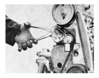
23. Remove the cross piece from the intermediate gear wheel. Check that cross piece is not damaged. Then remove the screw from the carrier. Use counterforce 999 5034. Remove the carrier and the pulley. Then remove the carrier from the pulley. Mild force from the rear with a wooden shaft or similar tool may be necessary.
