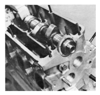
**114.** Oil and fit the last bearing cap. Then tighten all the nuts with a torque wrench. The tightening torque is 20 Nm (2.0 kpm) (14.7 lbf. ft.).
