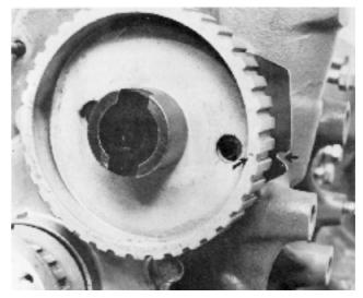
**124.** Turn the crankshaft into position after marking. Nick on the inner guide plate.
