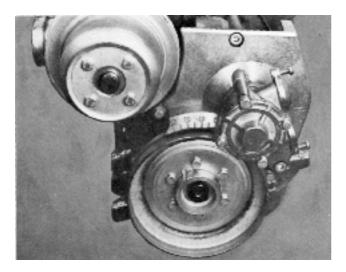
**161.** Fit a spacer ring and two sealing rings on the expansion tank's outgoing water pipe (1) and press in the tank's guide pin and pipes in the heat exchanger. The guide pin (2) is made of rubber. At the same time check that the support screw (3) has a plastic sleeve.
