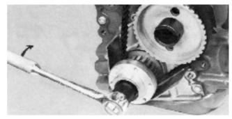
**130.** Loosen the nut on the belt tensioner againso that the spring tensions the belt. Check that the belt tensioner can move around its shaft. Then tighten the nut again. The tightening torque is 50 Nm (5.0 kpm) (36.9 lbf. ft.). Then rotate until the marking agrees for the crankshaft and check the marking for the intermediate shaft and the camshaft. The belt is to be tensioned once every season and to be changed every 500 hours.
