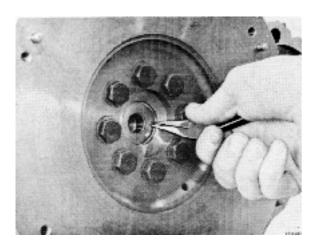
**56.** Remove the seal from the sealing flange with tool 999 2817.
