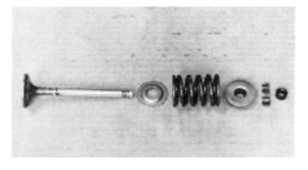
**38.** Remove the valves. Use valve spring compressor 884 580.
