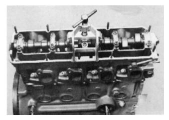
**112.** Lubricate the camshaft seal's rubber lip and fit it on the camshaft. Be careful so that the rubber lip is not damaged by the sharp edge when fitting it. Fit the sealing ring so that a new wear surface against the camshaft is obtained.
