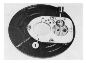
**92.** Disassemble the idling jet (1) and holder (2) for the main jet. Unscrew the jet from the holder. Blow the jets clean and replace if necessary. Unscrew the mixing screw (3) and blow clean the duct. Screw (4) locks tight the air cone (5).
