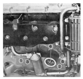
**156.** Lay a sealing ring on the heat exchanger's pipe (1) and press the pipe into the circulation pump and screw the heat exchanger to the exhaust pipe.
