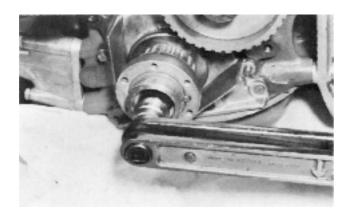
**125.** Turn the intermediate shaft into position after marking.
