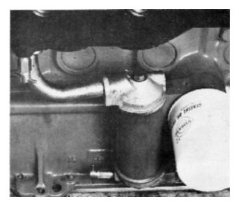
**10.** Remove the remaining three screws (X) on the heat exchanger and draw it to one side from the circulation pump.
