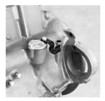
**135.** Fit a new rubber ring and gasket on the circulation pump. Fit the pump to the engine. Press the pump upwards against the cylinder head and tighten the screws and nuts.
