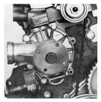
20. If the belt's markings have disappeared the belt is to be marked before it is removed. The marking of the belt is carried out as follows: Make a mark by the camshaft's pulley marking. Make a mark by the intermediate gear's marking and two marks on the crankshaft pulley's marking. Undo and remove the nut and washer for the belt tensioner.
