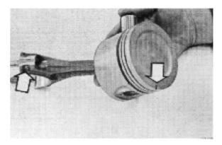
**100.** Fit the piston rings with piston ring pliers. The piston rings are to be fitted as shown in the picture. The upper ring is chromium-plated. The lower compression ring is marked "TOP". Turn the piston ring so that the gaps are at an angle of 120° from each other.
