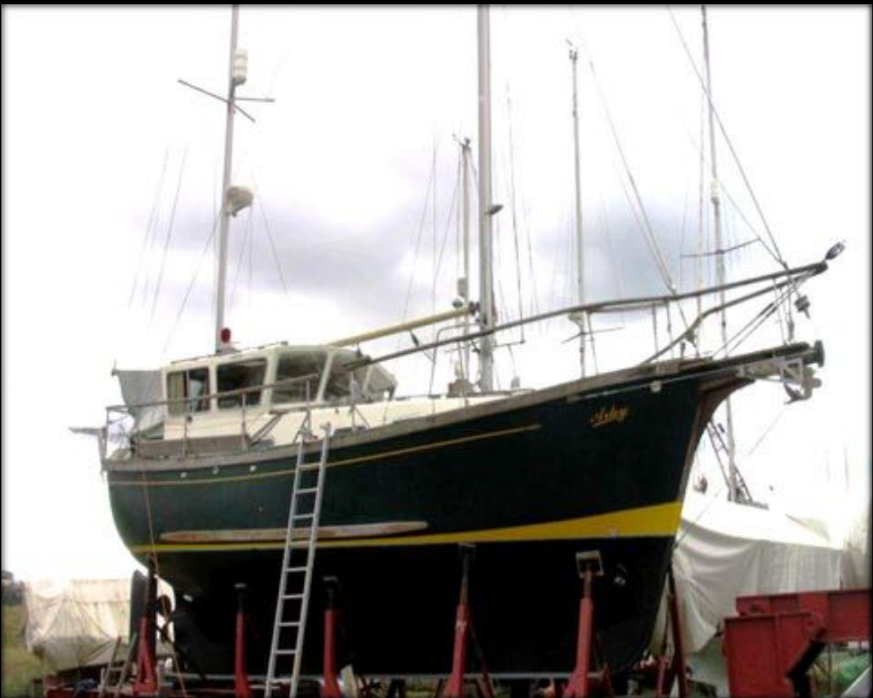
CW 34'-6" 'Arley' ashore showing that huge underwater hull and 4'-6" (1.37m) draft
