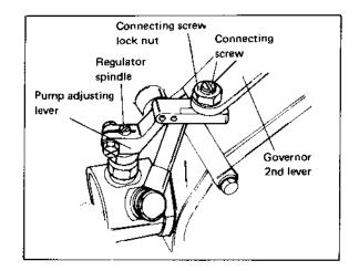
(2) Turn the punch mark on the connecting screw toward the cylinder perpendicularly to the pump adjusting lever.
