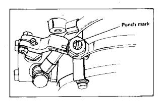
Note: If the pump adjusting lever moves outside when the connecting screw is turned by 90°, go back to step (3). After that, if the governor 2nd lever moves inside, the adjustment is perfect.
