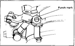
(Note) Drive in the connecting screw till its bottom comes to the top level of the pump adjusting lever.
