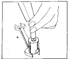
4) Take off the fuel injection valve spring holder, taking care not to drop the nozzle spring adjusting plates.
