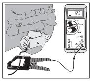
Figure 7: Measuring starter current draw Determine how much current the starter is drawing by using Fluke's i1010 Inductive Current Clamp on the starter cable. This accessory will allow the multimeter to measure starter current up to 1000 amps. Check manufacturer's specs for exact figures.
