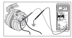
**Figure 5: Checking ripple voltage** Ripple voltage (AC voltage) can be measured by switching your DMM to AC and connecting the black lead to a good ground and the red lead to the "BAT" terminal on the back of the alternator, (not at the battery). A good alternator should measure less than 0.5 VAC with the engine running. A higher reading indicates damaged alternator diodes.
