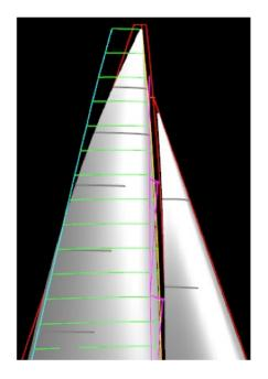
A moderate square-top main (light blue outline) can provide extra horsepower and a better twist profile, all for a relatively modest rating increase.
